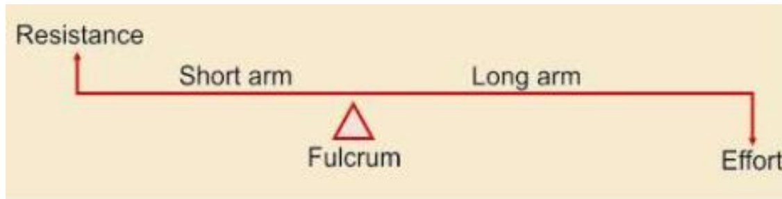
Fig. 5.19: Lever principle of elevation
