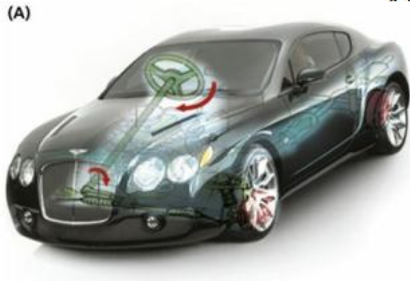
FIG. 17.16 Wheel and axle. x -radius of wheel; y -radius of the axle, E = effort, R = resistance, mechanical advantage of crossbar is
