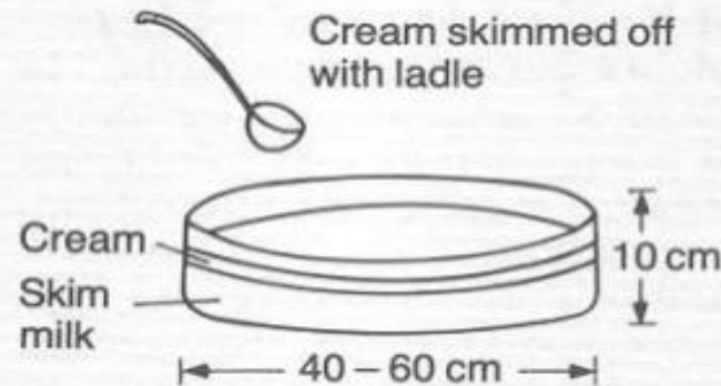
Figure 1. Batch separation of milk by gravity: (a) Shallow pan method, (b) deep-setting method
