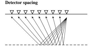
The reflection points on an interface will have a horizontal spacing equal to half the geophone/hydrophone spacing. By making this spacing **less than** the Fresnel zone, the survey resolution will not be limited by the layout, but by the physics of the wave propagation.
