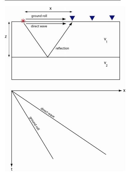
Seismic energy can travel from the shot (\*) to the receivers (geophones) by the 3 distinct routes shown in the upper panel. The lower panel is a **travel-time curve** and is a plot of travel time as a function of distance from the shot (x).
