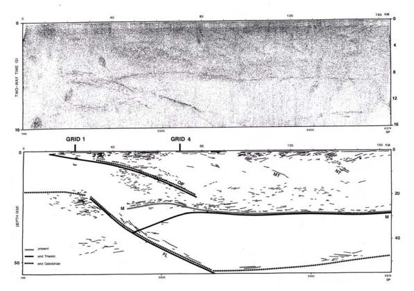
This BIRP clearly shows the Moho at about 8 seconds and a major thrust fault that apparently extends into the upper mantle. A common feature of many BIRPS profiles is significant seismic reflectivity in the lower crust. The origin of this feature is still not defined, but lenses of fluids, or mafic underplating are two possible explanations.
