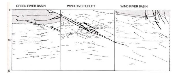
The figure above shows a seismic reflection image of the Wind River Thrust in Wyoming. This is a major feature associated with the Laramide orogeny (*Brewer et al*, 1980). Typical acquisition parameters for COCORP data were VIBROSEIS with a 96-fold CMP stack, recorder spacing of 100 m and spread length of 9.6 km. The VIBROSEIS signal was 8-32 Hz and at each location was stacked up to 80 times.
