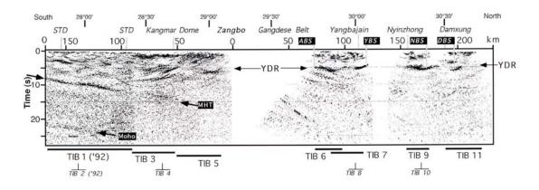
These seismic data imaged the Indian Plate being thrust beneath the Himalaya. The Main Himalayan Thrust (MHT) is the top of the Indian Plate. Note also that the Moho in the Indian Plate can be seen at a two-way travel time of 25 seconds. This observation showed that the 80 km thick crust was made by **stacking** Asian and Indian crust on top of each other (*Nelson et al*, 1996).
