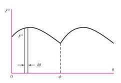
An example of this would be a cam whose bearings rotate with the cam through the angle  $d\theta$ . The total damage during a complete cam rotation is given by
