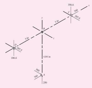
bearing is to be utilized at location *D*. The life goal of the speed reducer is 10 kh, with a reliability factor for the ensemble of all four bearings (both shafts) to equal or exceed 0.96 for the Weibull parameters of Ex. 11–3. The application factor is to be 1.2.
