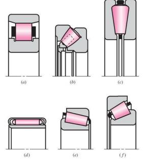
The spherical-roller thrust bearing (Fig. 11–3b) is useful where heavy loads and misalignment occur. The spherical elements have the advantage of increasing their contact area as the load is increased.
