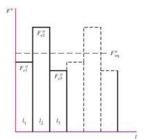
Consider the piecewise continuous cycle depicted in Fig. 11–10. The loads  $F_{ei}$  are equivalent steady radial loads for combined radial–thrust loads. The damage done by loads  $F_{e1}$ ,  $F_{e2}$ , and  $F_{e3}$  is
