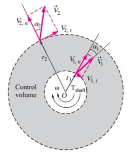
$\mathbf{T_{shaft}} = \dot{m}(r_2 V_{2,t} - r_1 V_{1,t}) \qquad \mathbf{T_{shaft}} = \dot{m}(r_2 V_2 \sin \alpha_2 - r_1 V_1 \sin \alpha_1)$
