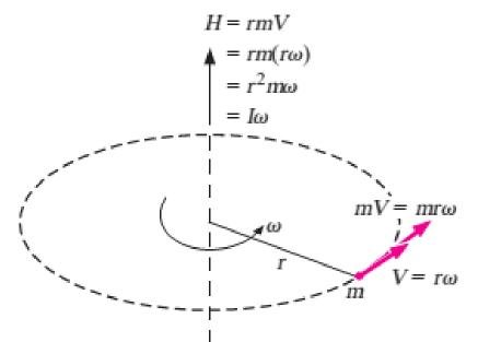
Angular momentum of point mass mrotating at angular velocity  $\omega$  at distance r from the axis of rotation. The angular velocity of rotating machinery is typically expressed in rpm and denoted by n., The angular velocity of rotating machinery is:  $\omega = 2 \pi N/60$  rad/s or
