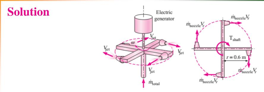
The conservation of mass equation for this steady-flow system is  $m_1 = m_2 = m_{tot.}$  $m_{nozzle} = m_{tot.}/4$  or  $\dot{V}_{nozzle} = \dot{V}_{total}/4$
