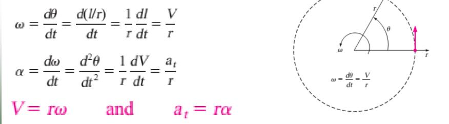
V is the linear velocity and  $a_t$  is the linear acceleration in the tangential direction for a point located at a distance r from the axis of rotation.
